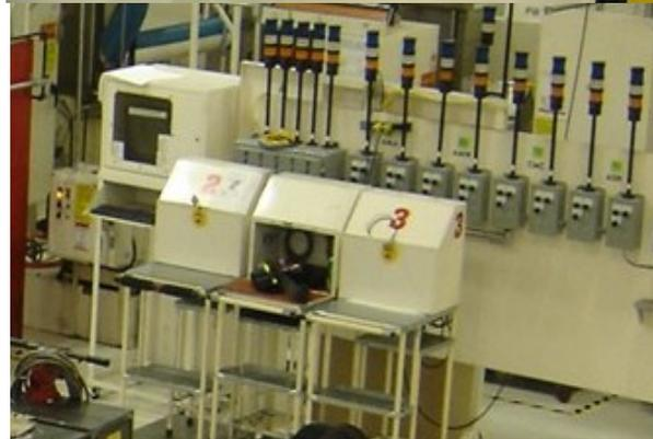
Maintenance and engineering areas adjoin the shop (top) with three machine debugging carts stationed near the andon lights at upper right. Each plant area has an andon light stack. Each cart (bottom) has identical laptops, diagnostic software, and the cables for plugging into any machine. The laptops use the plant’s wireless network so electricians can download machine programs from a database or research and order parts from the internet.
