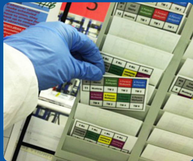
Boxes on cards tell the observer what Cell and operation to check, depending on which of three possible takt times are in effect.
