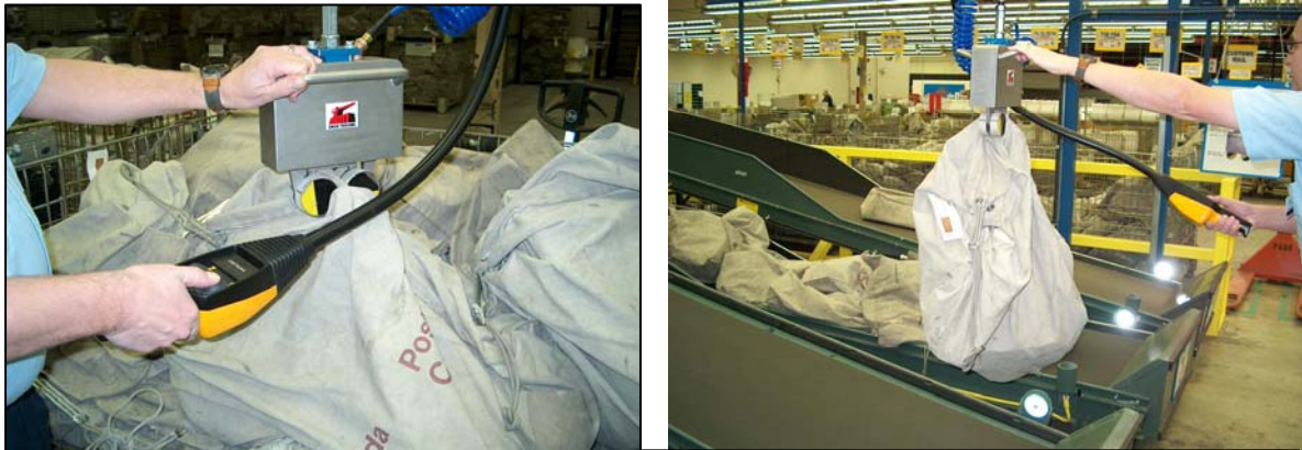
An operator at the induction station uses a lift assist arm to remove a mail bag from a cage and place it on a belt leading to a workstation where another operator will open it and sort the contents.
