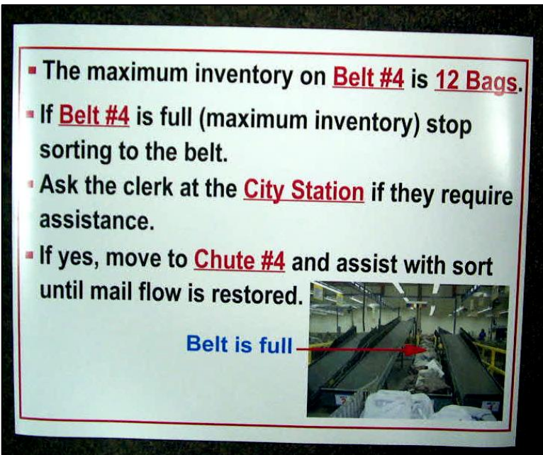
A standard work document at the pubs and ad mail cell tells operators how to respond to a spike in volume at the sorting station for Calgary mail.
